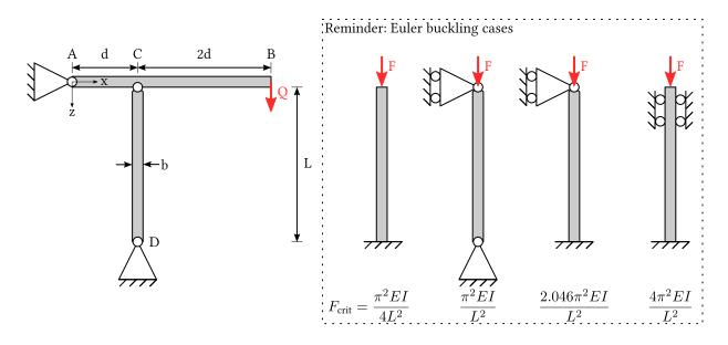
**Solution:** We first need to compute the normal force F in column CD. We cut the two members at point C. The equilibrium conditions yield
