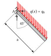
**Solution:** To find the resultant of the line load, we need to integrate along the length of the beam. For this purpose, we introduce a coordinate system whose x'-axis is aligned with the beam axis and split the line load into parallel and perpendicular components  $q_N(x')$  and  $q_Q(x')$ , respectively. Considering the angle, we obtain
