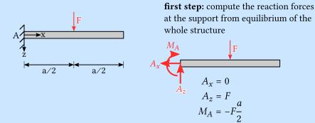
second step: divide beam into sectors and compute internal forces
