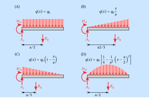
A beam of length a is mounted on the wall at an angle of 45°. A constant line load  $q_0$  is applied. Calculate the reaction forces and the bending moment about the y-axis at point A!
