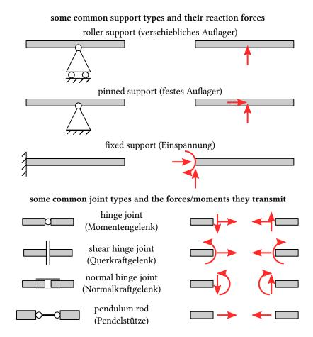
Recall that a 2D structure is statically determinate if
