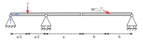
**Solution:**  $n = 2, r = 4, v = 2, \quad 3 \times 2 - (4 + 2) = 0 \implies$  the structure is statically determinate. We will cut the girder at the hinge and require equilibrium for each of the two bars. Keep in mind that  $\sin(30^\circ) = 1/2$  and  $\cos(30^\circ) = \sqrt{3}/2$ .
