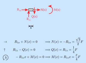
We will cut the bar right of the point where F is applied and require equilibrium for this section to determine the internal forces and moment there:
